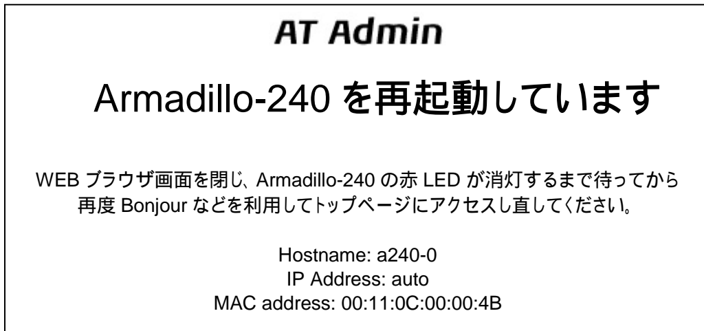
図 5-12 AT Admin: System – Reboot
